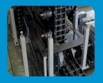
**The solution:** Linear Chain with special profile interlocking fingers that allows it to become a rigid thrust device for pushing a guided load.
